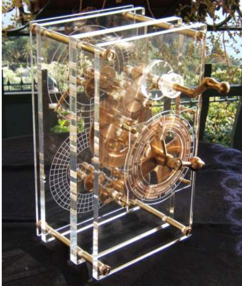
A 2007 mechanical model based on the ancient Greek Antikythera machine. (Photo by Mogi Vicentini, WikiCommons)
