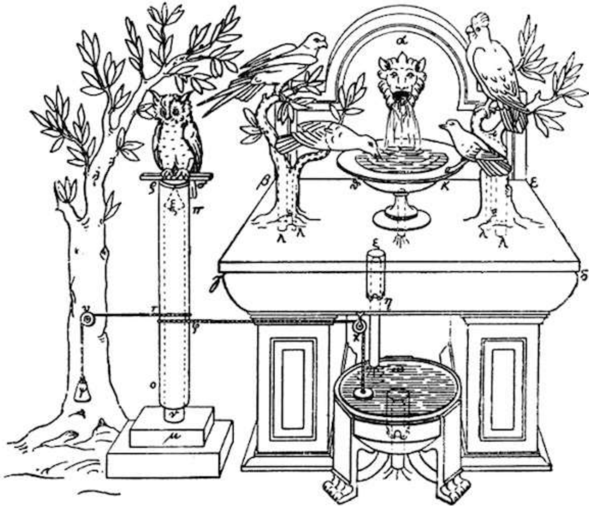
This sketch, based on Hero of Alexandria's writings describing water- and weight-driven bird automata, appeared in Sigvard Strandh's 1989 book, The History of the Machine .
